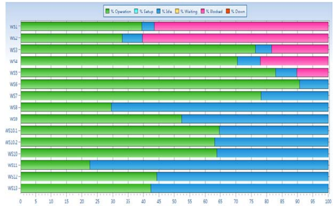
Fig. 3: Work Station Utilization before balancing.
