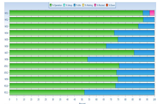
Fig. 4: Work Station Utilization after Balancing
